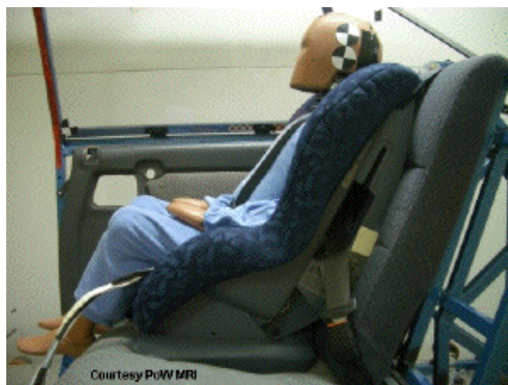
Figure 13. Illustration of less favourable geometry with inclined seat and child
