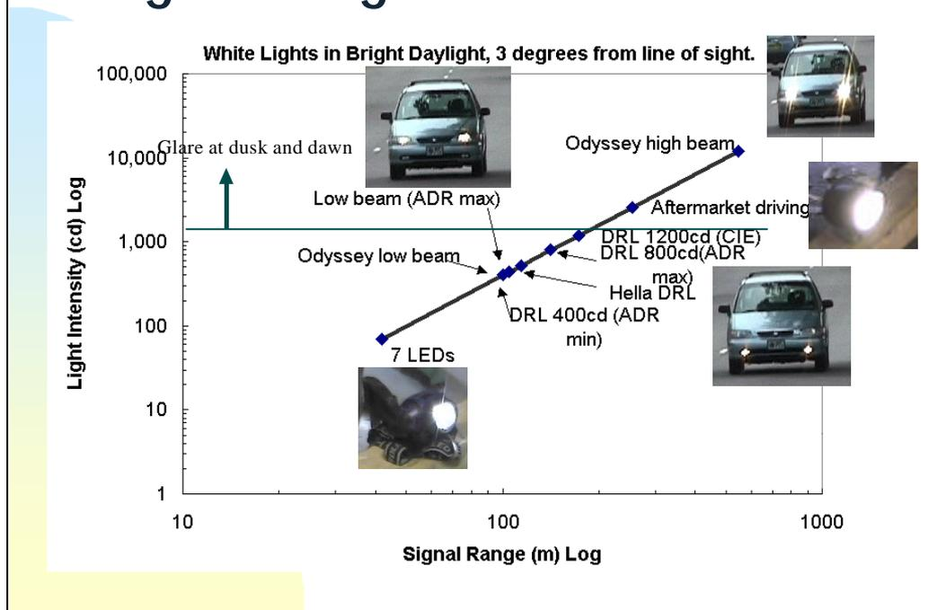
This graph shows the signal range in bright daylight for a range of potential white DRLs. I have switched to a log-log plot to cover the large range.
