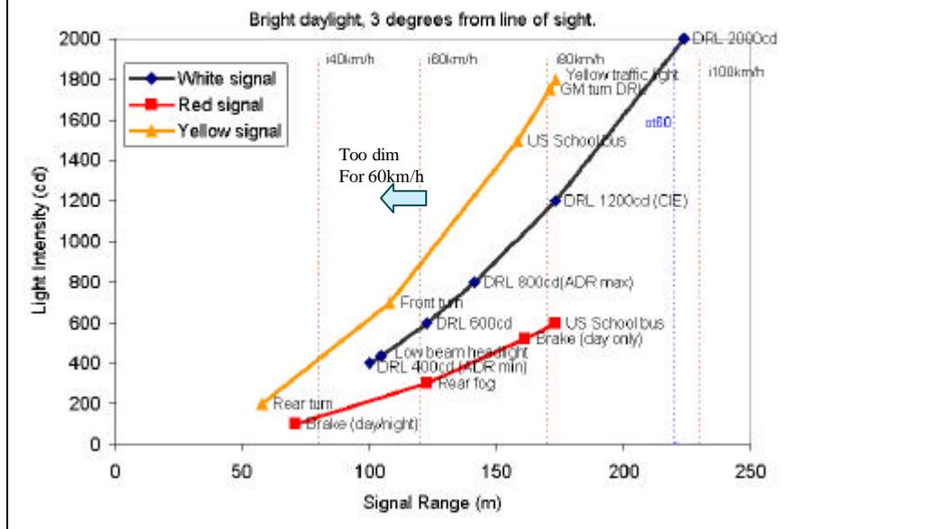
Applying some typical road conditions gives these signal ranges for a selection of vehicle lights of various intensities. This graph appears in my research report for the NRMA and RACV.
