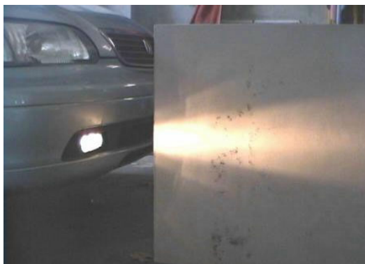
Vertical and horizontal distribution of beam
