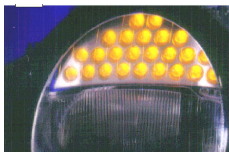
Figure 5. Prototype turn signal lamp with high intensity LEDs (from Decker 2000)
