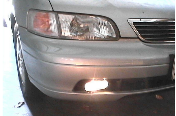
Installed dedicated DRL
