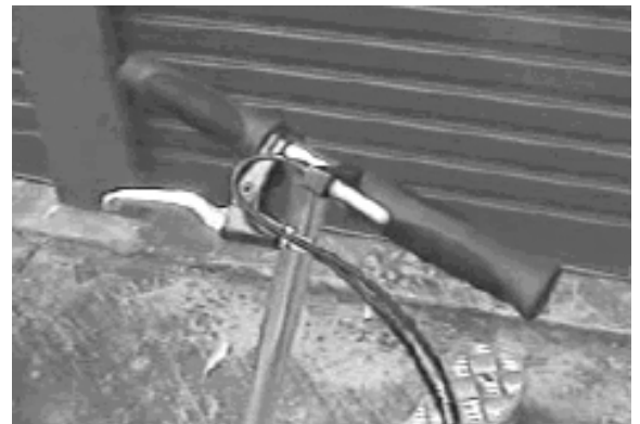
Hand levers - large lever is brake. Short lever is throttle (on/off).
