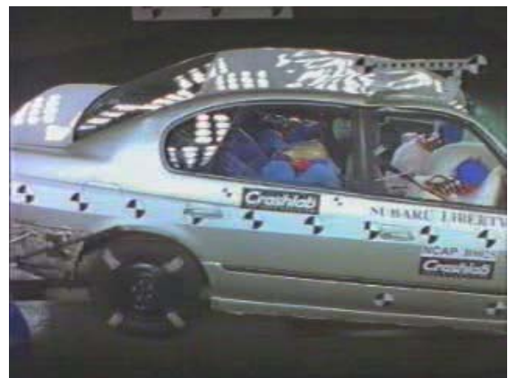
Figure 7. ANCAP Offset Frontal Crash at 64km/h
